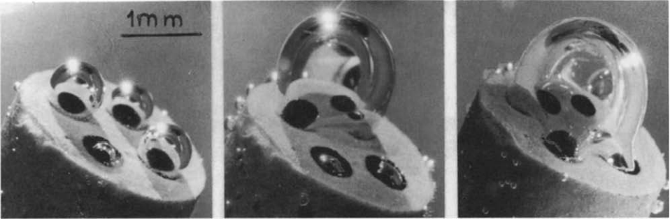
Fig. 8. Hydrophobic areas on a hydrophilic base. Immersing the model into air saturated water, gas accumulates on the hydrophobic parts of the surface. The gas accumulations are first lenticular, then half spherical bubbles. Further gas diffusion into the bubbles enlarge them causing a distortion. If one bubble comes into contact with its neighbour they unify into a larger, even stronger distorted bubble that clings to several unwettable plinths on the wall. Due to the deviation of shape of the bubbles from being spherical and resulting distortion of the bubbles the bubble bearing wall must be stressed by equivalent forces (see Fig. 9 and 10).
