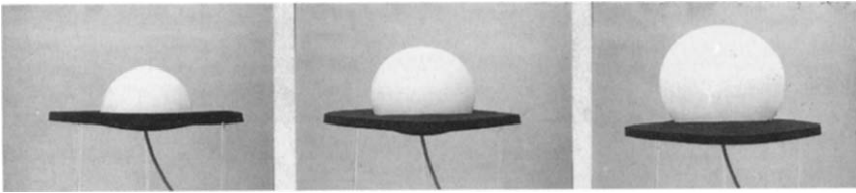
Fig. 9. A rubber balloon which is half spherical and inflatable is attached to an elastic rubber plate. (A taut rubber membrane has a similar behaviour as a liquid surface.) The line of contact of the membrane to the plate cannot alter, just as a gas bubble that clings to a hydrophobic plinth. When overstretching the balloon by a high internal pressure results a distortion of the plate with a slope toward the pole of the balloon.
